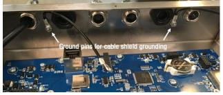
**Warning**: Incorrectly closed back cover and poorly tightened glands may be unwanted results with loss of IP rating and safety. Tighten the glands' cup nut with minimum 5Nm torque.
