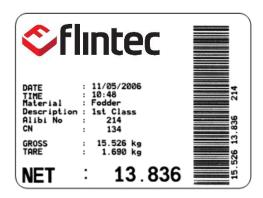
Figure 7.1- Sample of the label printout of FT-111 which is designed in EPL format.
